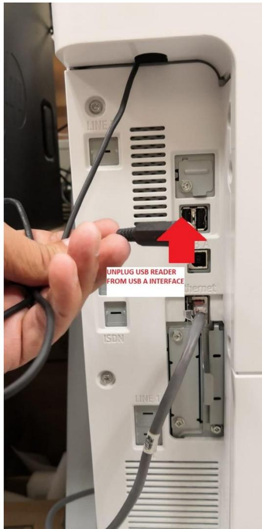
Depending on model, card reader cable should be guide inside Ricoh device. In that case you should open back cover and remove USB card reader cable.
