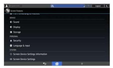
Press IC card/ Bluetooth software settings → Select IC card reader →Proximity card reader For IMC Devices option is External Interface Software Settings
