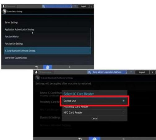
Once enabled a new menu "Do not Use" will appear. A message to connect the card reader will pop up. As specified above, the card reader needs to be connected to one of the USB ports on the Operation Panel.
