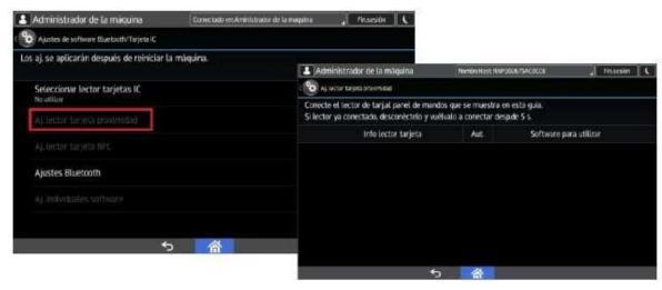
Once the card reader is detected by the system, the menu can be closed, after that, a physical <u>restart</u> of the device is mandatory; if it is not done the card reader cannot be recognized.
