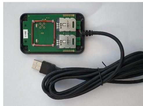
Push down on top of the reader housing while slightly moving it towards the cord.
