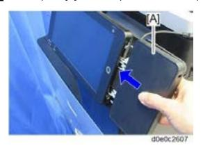
**<u>11.</u>** Insert USB cable [A] into the connector on the operation panel.
