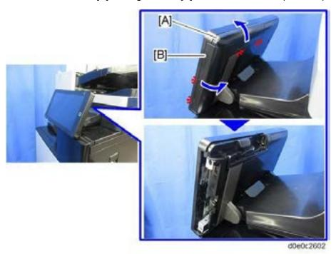
**10.** Insert option [A] into the option slot on the operation panel.
