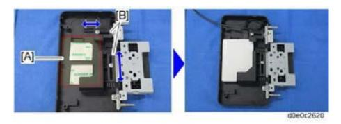
5. Attach fastener [B] about 16 cm (6.3 in.) [A] from the end of the USB cable. Use the vertical length of the optional cover as a guide.
