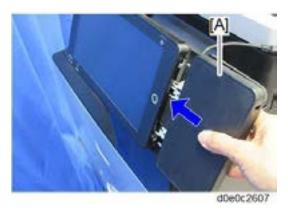
11. Insert USB cable [A] into the connector on the operation panel.
