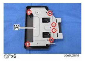
3. Attach sponge cushions [A], and then adjust brackets [B] to the card reader spacer, if necessary.
